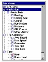
Overlay Data with Navigation, Trip Calculator and Time categories expanded.
